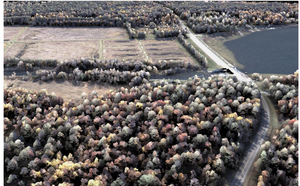
Lidar point cloud colored by photograph pixel colors
